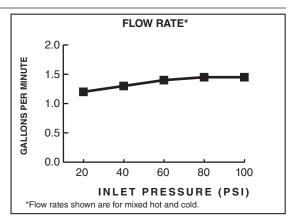
1.5 gpm/5.7 L/min. FLOW RATE
