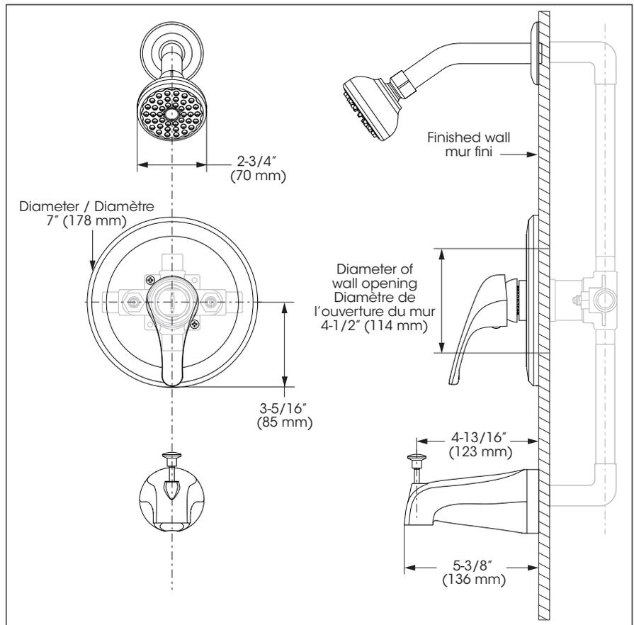
Bathtub / Shower Faucet (T/P) – Trim for Thermostatic Pressure Balanced Valve with Volume Control
