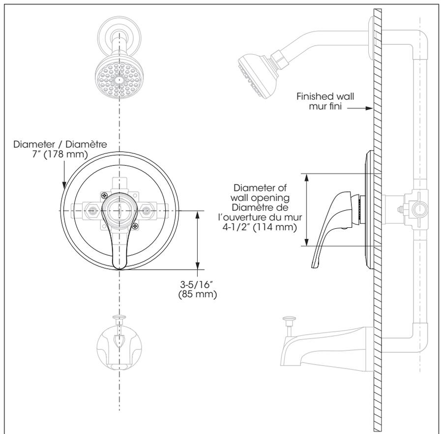
Trim (T/P) for Pressure Balanced Thermostatic Valve
