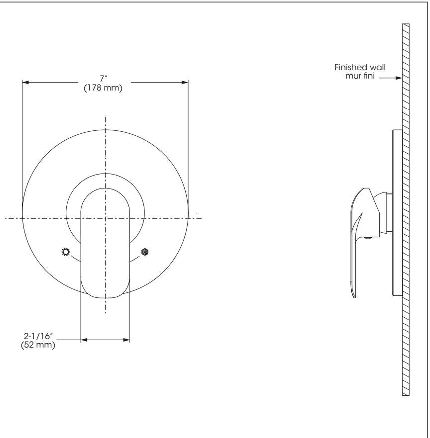
Valve - Trim for Pressure Balanced Diverter Valve with Volume Control
