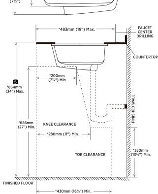
NOTE: \* Starred measurements comply with CSA B651 and OBC barrier free accessibility requirements.
