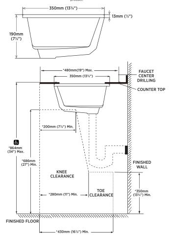
NOTE: \* Starred measurements comply with CSA B651 and OBC barrier free accessibility requirements.
