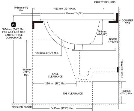
**NOTE: \*** Starred measurements comply with ADA and OBC barrier free accessibility requirements. **\( \Delta\)** Dimensions shown for location of supplied and waste are suggested.
